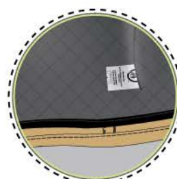
Heat barrier is fastened to outershell fabric with snap buttons
