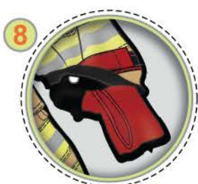
Anti-wicking tapes on sleeve hems to prevent water absorption
