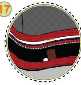
Anti-wicking fabric to prevent fluid entry Water drain holes Inspection opening with zipper closure
