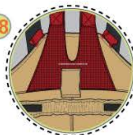
Velcro tapes for belt of full body harness
