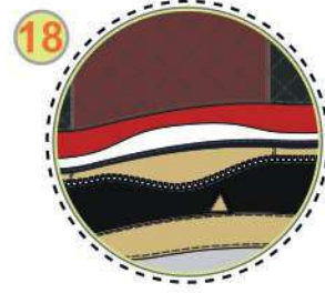
Anti-wicking fabric to prevent fluid entry Water drain holes Inspection opening with zipper closure
