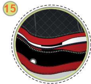
Anti-wicking fabric to prevent fluid entry Water drain holes Inspection opening with zipper closure
