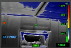
**Find hidden heat sources during overhaul.** Patented technology empowers users to throttle sensitivity up and down to visually isolate warmer items in any type of scene.
