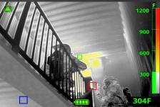
**Save time with instant info.** Instantly identify the hottest area of the scene with Hot Area Detector. Use Cold Area Detector to find the coolest spot on-scene. Zoom
