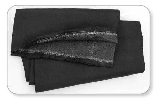
Fabric: 192062012 CF W-2000Outer Surface: Carbon (Black)Reinforcement Layer: Glass Fiber Fabric (white)
