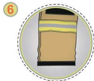
Trotter reinforcement and yellow - silver - yellow reflective tapes
