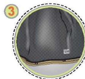
Heat barrier is fastened to outershell fabric with snap buttons
